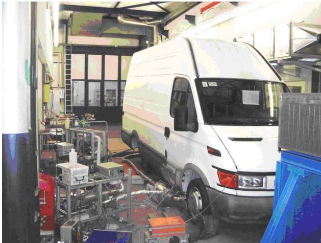
Empa ICEL, test bench, Bach & al., SAE 2011-24-0179
