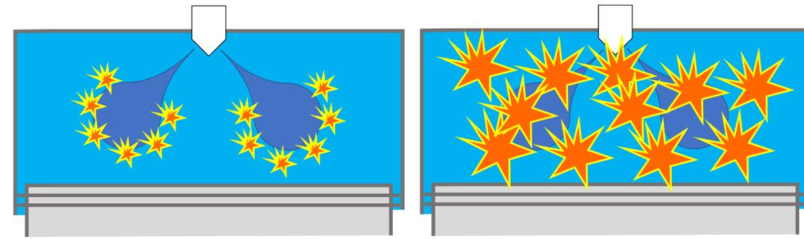
Cold injection must produce an almost homogeneous mixture
