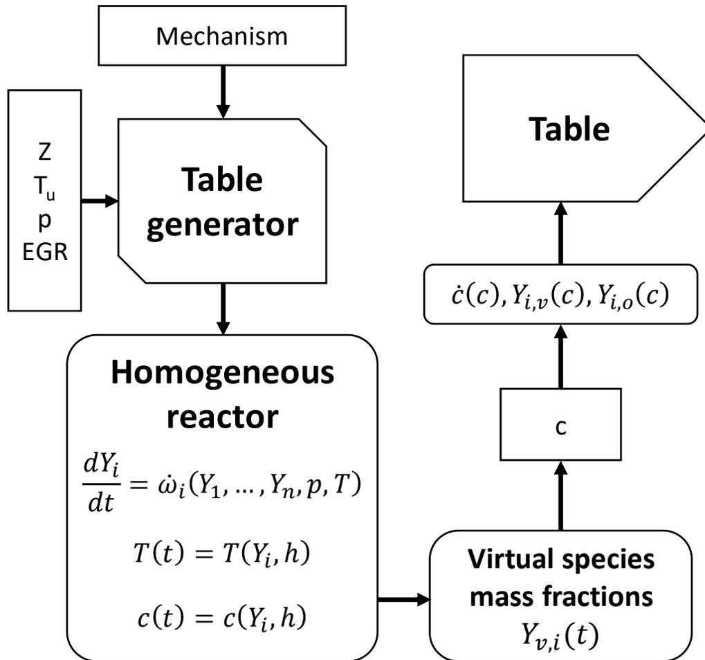
CFD solver: tabulated kinetics ensures reduced computational time and results accuracy:
